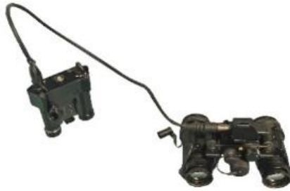
Figure 11 External Battery Pack Interconnection
