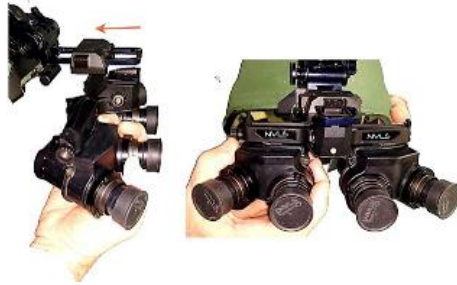
Figure 12 Installing PD-PRO-Q on Helmet Mount
