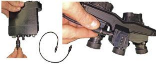
Figure 13 Connection Power Cable
